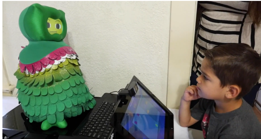
Figure 1.1: Socially assistive robot system setup used for improving social and cognitive skills of students on the autism spectrum, evaluated in month-long in-home deployments (Shi et al. 2022; Clabaugh et al. 2019; Clabaugh et al. 2020; Jain et al. 2020a; Pakkar et al. 2019).
