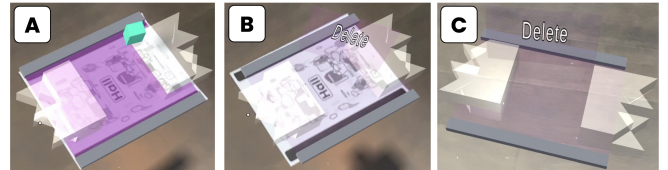
Fig. 5: All possible states of tracking a piece of maze paper. A) Tracking & In View: virtual analog is overlaid with spinning tracking indicator cube; B) Not Tracking & In View: virtual analog persists having higher transparency, removing the spinning indicator cube, and adding a delete button; and C) Not Tracking & Not In View: virtual analog is identical to B.
